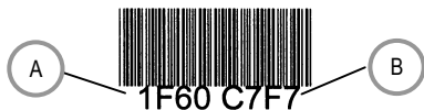
Figure 45: Sensing Head Calibration Data printed on the Cable (e.g. Head with two blocks of 4 numbers)
